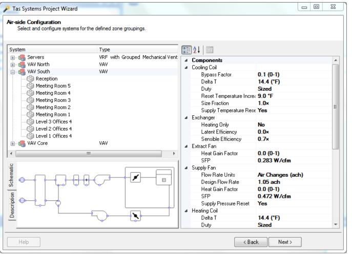
This building has four air handling units. Three VAV systems serve South facing areas, North facing areas, and core areas. Server rooms have cooling from local VRF units, with common mechanical supply and extract.
